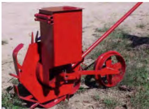
This machine punches holes and deposits one or more grains in it. The holes have a medium fixed distance of 23 cm.
