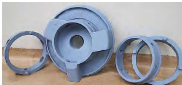
Seed distribution is done with a rotating ring, which catches the grain in its six holes, and delivers it to the beaks of the wheel.
